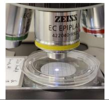
In Particulate Contamination Testing applications, MML customers are seeking to determine the quantity of unexpected and/or unwanted contaminant particles present in or on the surface of the sample. A combination of automated particle counting instrumentation (LO) and optical microscopy (MM) is used for these applications.
